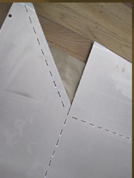
Flat CNC cut aluminum sheet with folding perforations
